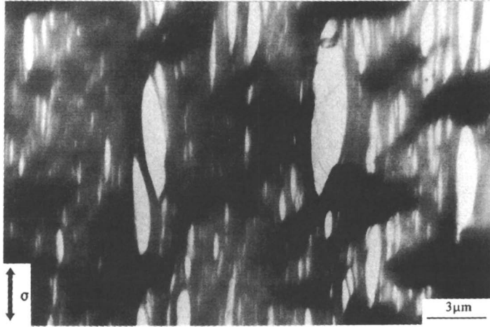
Figure 13. Highly deformed, toughened PP, showing cavitation inside the particles and intense plastic deformation of the matrix strands (HVEM image). The deformation direction is vertical.
