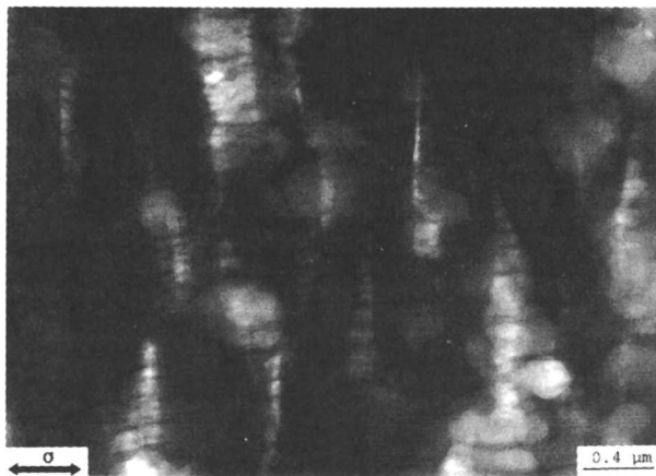
Figure 4. Crazes originating at rubber particles, with some partly ending in the matrix (HVEM image). The deformation direction is horizontal.
